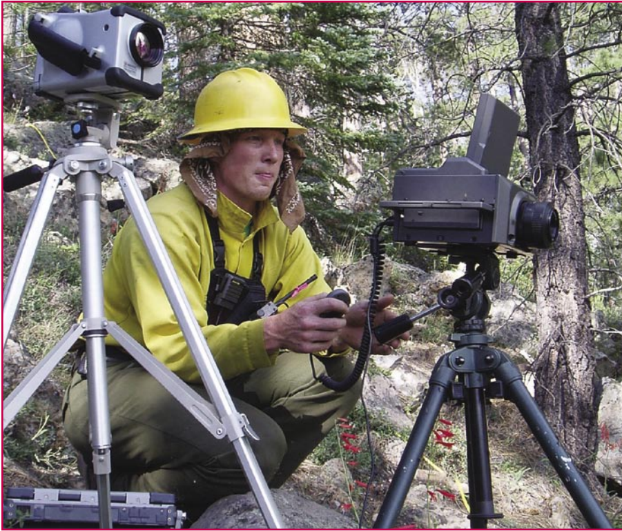
Thermal Infrared—Patrick Freeborn, physical scientist with the Fire Chemistry Research Work Unit, Missoula Fire Sciences Laboratory, Missoula, MT, operates both mid- and short-wave thermal infrared cameras to monitor radiant heat flux and temperatures on the Dragon Complex Wildland Fire Use Incident on the North Rim of the Grand Canyon, AZ. Freeborn installed these cameras inside the Rapid Response Research plots. Photo: Colin Hardy, Forest Service, Rocky Mountain Research Station, 2005.
