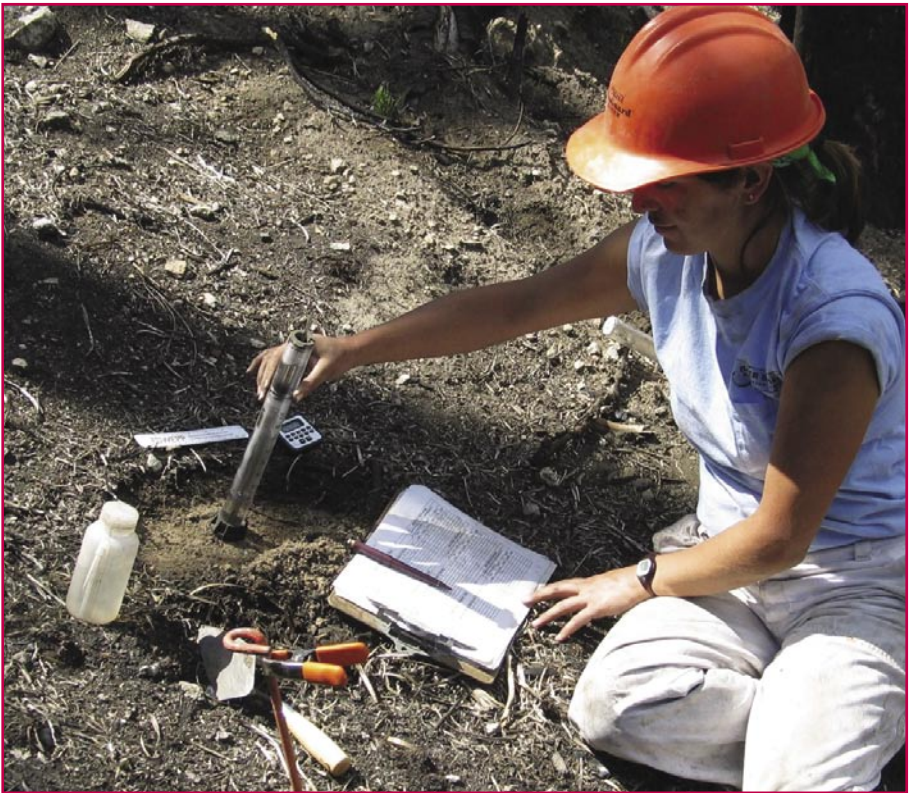
Measuring Water Infiltration Rate—Sarah Lewis, civil engineer with the Soil and Water Engineering Research Work Unit, Forestry Sciences Laboratory, Moscow, ID, measures relative water infiltration rate to assess the degree of post-soil water repellency after the Hot Creek Fire on the Boise National Forest. Photo: Pete Robichaud, research engineer, Forest Service, Rocky Mountain Research Station, 2005.
