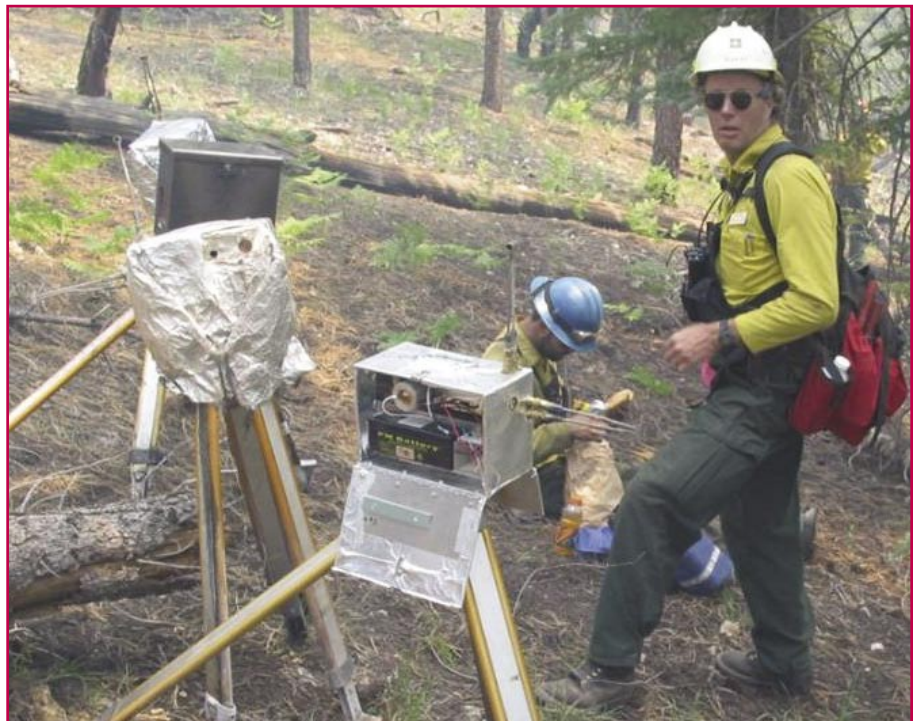
Feel the Heat—Fire-protected video systems and instrumentation for measuring heat flux, fire behavior, and local weather are installed on the Dragon Complex Wildland Fire Use Incident on the North Rim of the Grand Canyon, AZ, by mechanical engineer Jason Forthofer (sitting) and project leader Colin Hardy. Both men are from the Fire Behavior Research Work Unit, Missoula Fire Sciences Laboratory, Missoula, MT. Photo: Dan Jimenez, Forest Service, Rocky Mountain Research Station, 2005.
